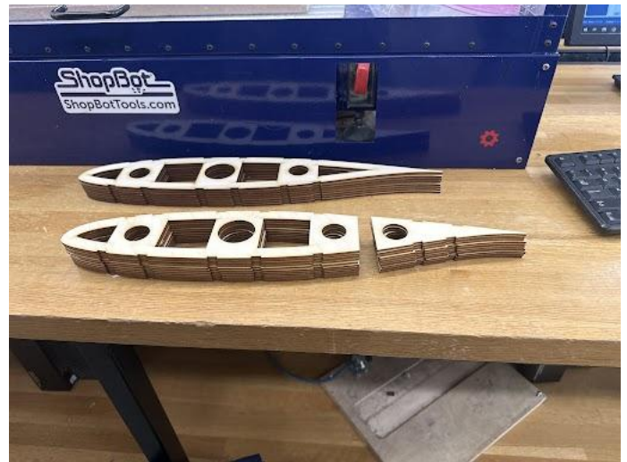
Figure 2 : Airfoil Cross-Section Manufactured
